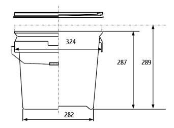
Measurements in millimetres
